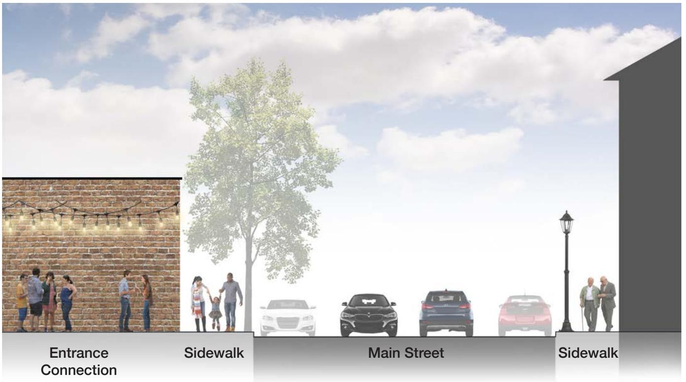
Figure 1-11: Section 2: Typical Road Cross Section Parking on Both Sides
